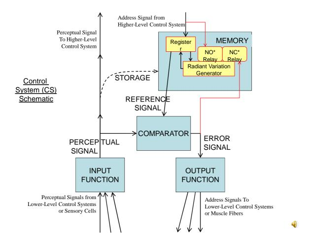
As long as an address signal is being received by Register r from a higher level Control System (CS) (subject to the actions of the two relays\*) the Radiant Variation Generator copies the reference signal stored in Register r, modifies some of its elements slightly, at random, and stores the modified signal back in Register r; whereupon, of course, the new reference signal is copied into the comparator and the sequence repeats.
