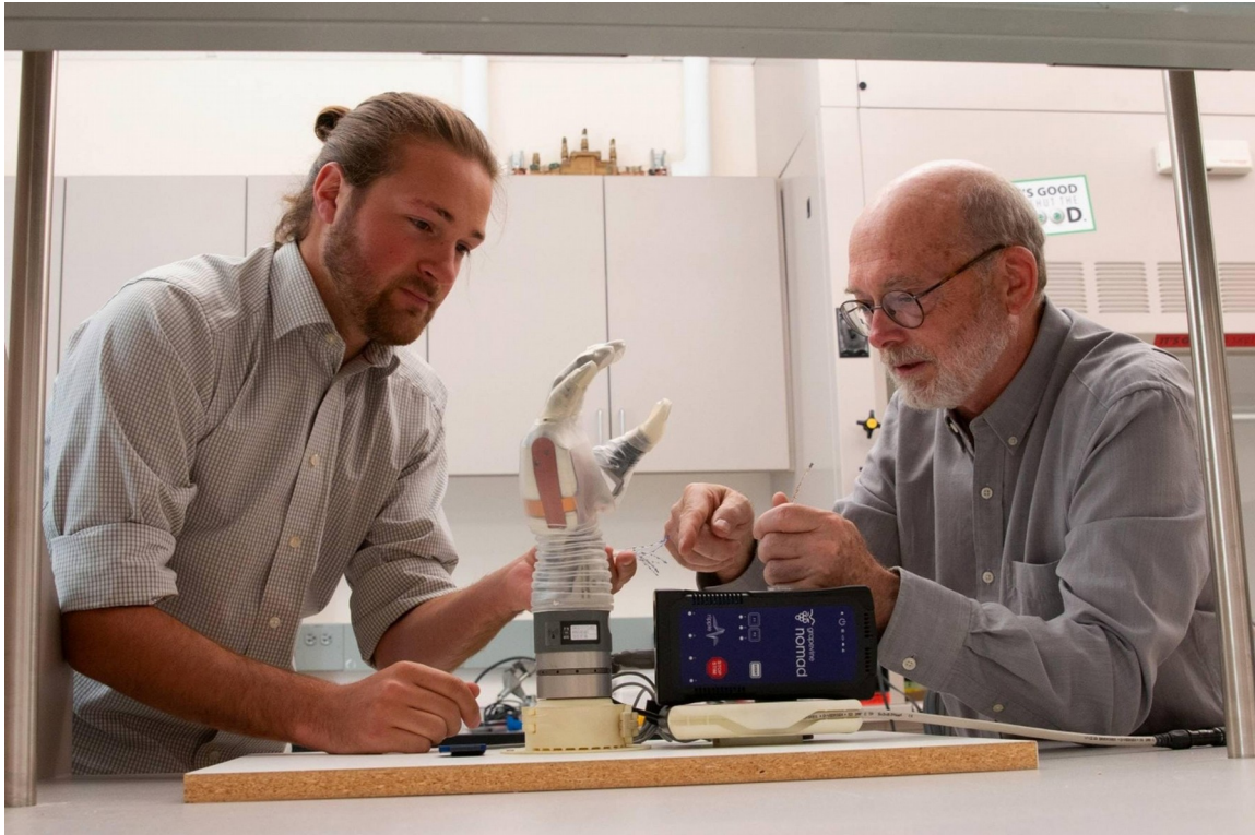
Doctoral student Jacob George, left, and professor Greg Clark examine the LUKE Arm, a motorized and sensorized prosthetic that has been in development for over 15 years. (Dan Hixson/University of Utah College of Engineering)
